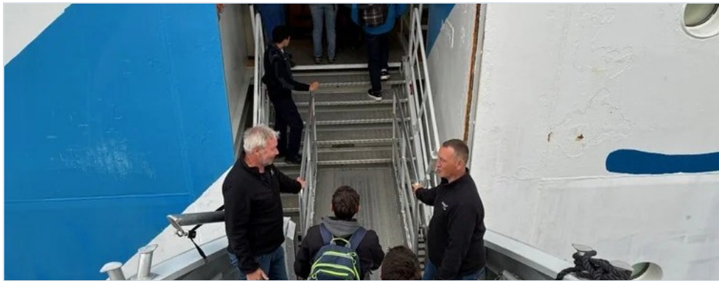
Holly’s bow lobby mated with an AIDA vessel’s shell door – guests walk straight through, two Holly crew supervising.
